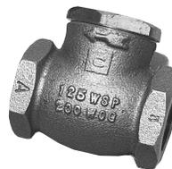
**Gas check valves** should be horizontally installed in multi-burner applications as close as possible to each burner inlet for dependable light-off (gas manifold may otherwise act as a reservoir, preventing light-off during trial-for-ignition period).
